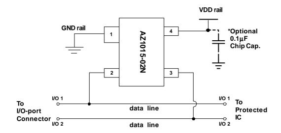
Fig. 2 Data lines and power rails connection of AZ1015-02N.
